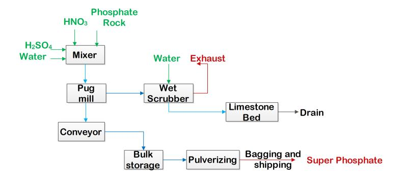
Figure: Manufacturing of Superphosphate by nitric and mixed acid acidulation
